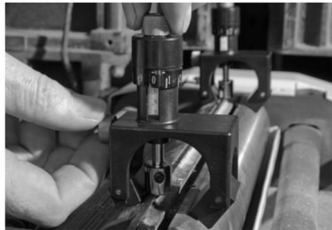
**1.** Place both Jigs on the cutter block surface and check they are both Synchronised (i.e. they both read the same measurement on the scales), see top picture.
