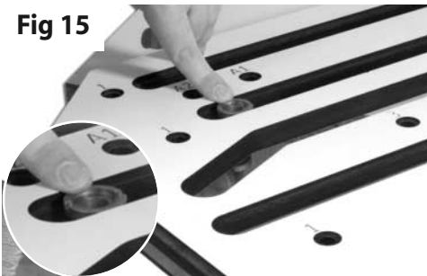
Fig 15 Fitting the Dowel pin Locator in to the 'S' slot
