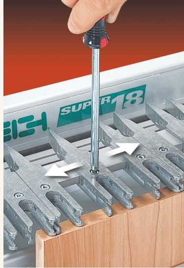
▲ **Fingers.** To customize the size and spacing of the dovetails, just slide the fingers into position and lock them securely in place.
