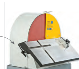
Adjustable tilt work table mounted on strong trunnions
