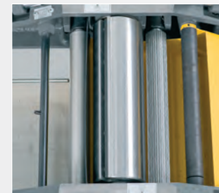
Three-knife cutter block gives a very clean finish to the work
