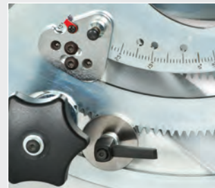
Quick angle index system for most common tilt angles
