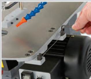
Articulated hose provides air from a bellows
