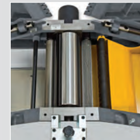
Four HSS resharpenable knives
