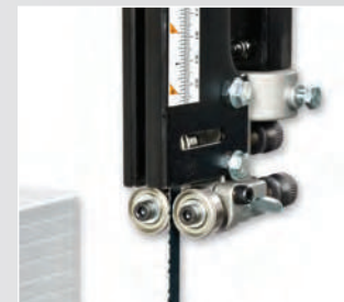
Micro adjustable ball bearing blade guides, easy to set
