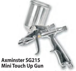
A handy little spray gun, useful for spraying small areas of work or modelling projects. Can handle almost all finishes including water based acrylic enamels. Easy to use and comfortable, especially in the smaller hand. Fitted with a stainless steel paint flow needle, air fan control, paint regulator and 125ml suction feed cup. 1/4" BSP male inlet fitting. Takes quick release bayonet fitting 100314 or 410250 (swiveling).
