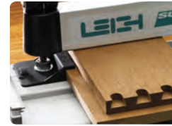
Under cut side stops for rabbeted drawer fronts
