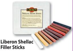
Traditional sticks of coloured shellac in ten assorted shades. Used to fill holes or make repairs prior to French polishing, lacquering or varnishing. Melt the sticks into the blemish using a hot iron. It dries very hard and should be levelled with fine abrasive. Each stick is approximately 85mm long and 10mm diameter.
