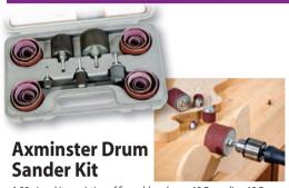
A 25 piece kit consisting of five rubber drums: 12.7mm dia x 12.7mm long, 19mm dia x 25mm long, 25 mm dia x 25mm long, 38mm dia x 38mm long, 50mm dia x 38mm long and supplied with fixed diameter sanding sleeves in 80 and 120 grit. Endless uses and a real must for anyone's tool kit. Max speed 1500 rpm. Supplied in a plastic case.
