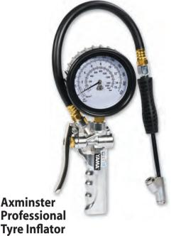
This is a rugged tyre inflator with a dial reading pressure gauge, more like the one you find at the local garage (or maybe even better!). With a large, clear gauge protected by a rubber housing, it reads in psi, kg/cm<sup>2</sup>, kpa and bar. Cleverly, the gauge swivels to allow left or right handed use. It has a 1/4" BSP female fitting. For quick release couplings use 100313 or 410251 (swivelling).
