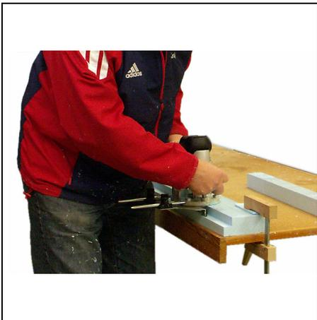
Mould rebates on roof, door, sill and sidewalls of the kiln.
