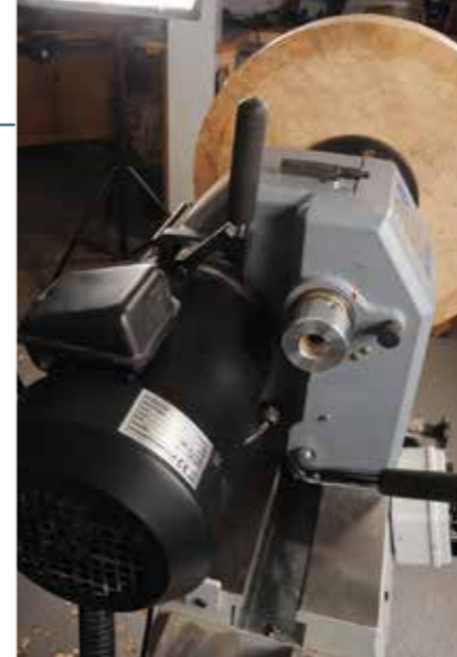
The back end of the headstock casting showing motor assembly, indexing, headstock lever locking handle and bed extension in a lower position
